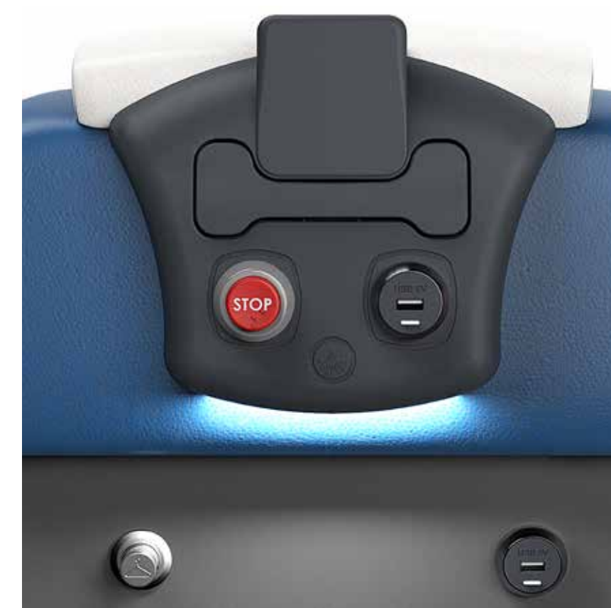
Console with usb, bell push, led reading light, smartphone holder with/without wireless charger
